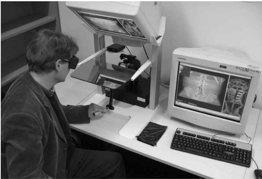
**Fig. 9** One of the co-authors using the virtual lumbar puncture trainer wearing shutter glasses to enable stereographic visualization.
